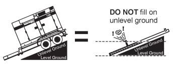
Figure 29. Only Fill on Level Ground
